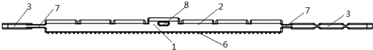
**Illustration 2:** *In order for the machine to work, make sure that the USB Chord is properly connected to the USB connector (8) on the side of the device.*
